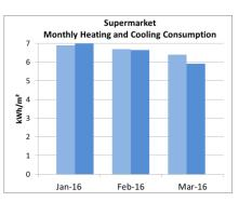
consumptions in the North and West perimeter zones were also lower by over 17%. It was only slightly sunnier than the average but the cooler air temperature is beneficial to the PV panel efficiency and therefore the PV model had an encouraging energy yield that was 6.3% higher than the average.
